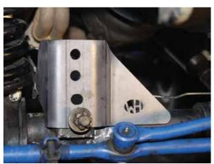
Using stock bolt to line up bracket for track bar positioning
