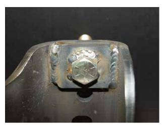
Welding support bracket and bolt
